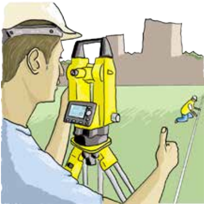
Surveying theodolite construction ground settlement measuring work.png
